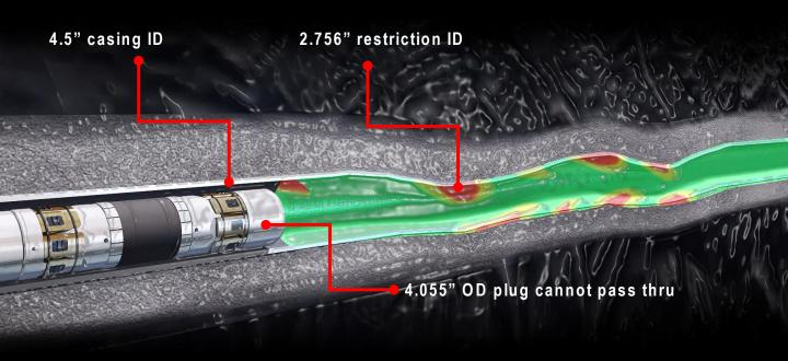
Since 2016, Vertechs has been developing and offering high-expansion dissolvable frac plugs to address downhole restrictions. These plugs are designed to save untreatable stages and speed up completions by providing a solution for challenging restrictions.
